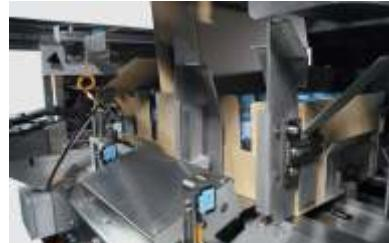
During descent of the products, the flat carton blank is wrapped tightly around the products in just one step. This leads to a rigid and safe transport case. The use of partition boards can be avoided in most applications. The accurately aligned tight cases or trays guarantee optimal stacking when palletized.
